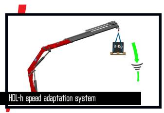
HDL-h is an electro-hydraulic system which automatically adapts the crane speed to the working situation. You thus avoid big and sudden stress, which may damage the crane or influence the stability of the vehicle in an unfavourable way. The RCL 5300 is monitoring which movements that have to be adapted.
