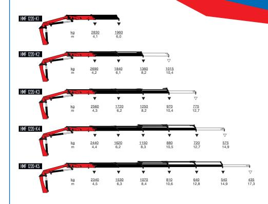
▼ Lifting capacity without manual extensions✓ Lifting capacity with manual extensions
