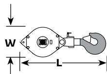
► **Hook block for 26 mm (1 inch) wire rope**
