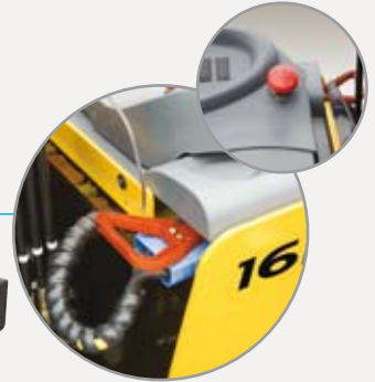
Battery Disconnect Lever & Emergency Switch
