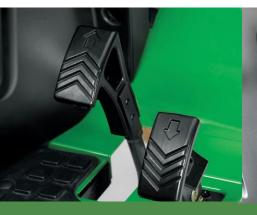
Twin Touch™ transmission pedals make it easy to switch from forward to reverse, and let you rest your heel on the platform the whole time you drive.
