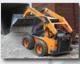
VERTICAL-LIFT A design delivers extended reach and 131-inch lift height, higher than any competitor in its weight class.
