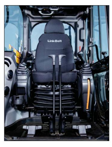
The X4 Series offers one of the most advanced and roomiest cabs in its class. Comfortable, automotive-grade high-back seat with head rest provides superior lumbar back support. With a longer and wider seating surface, it reclines to a 155° maximum reclining angle to create a relaxed environment during breaks. Air-suspension seat is standard with tilting adjustment and seat heaters available as options.
