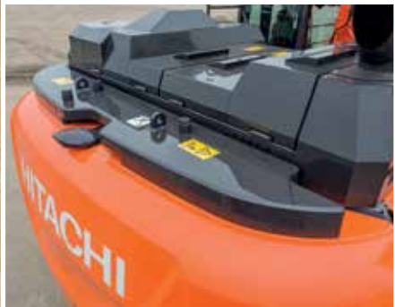
The smaller additional counterweight makes it easy to handle and improves safety.
