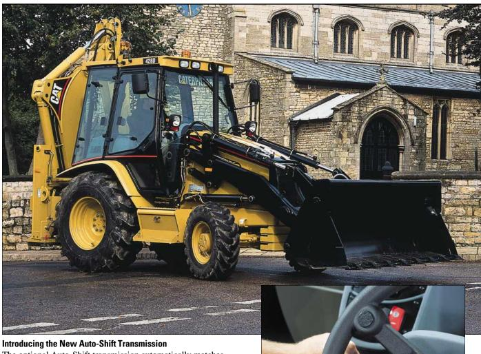
The optional Auto-Shift transmission automatically matches gears with grade and load conditions.
