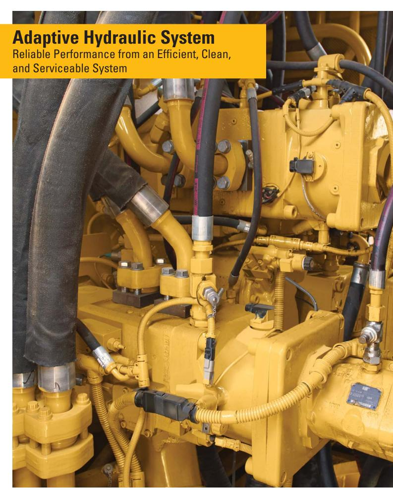
The revolutionary Adaptive Hydraulic System combines industry-leading and patent-pending dedicated pump-flow allocation technology with proven Cat features like independent oil cooling and boom float to generate flow and pressure, without waste – providing a 20% fuel efficiency advantage.
