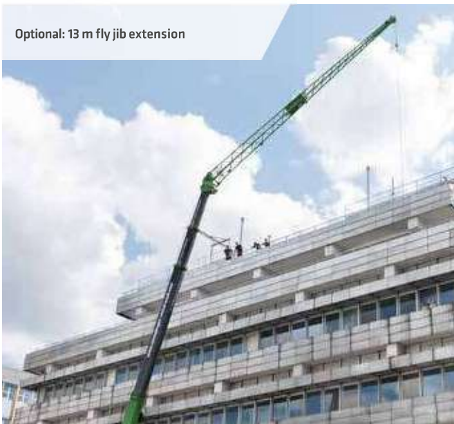
Fly jib incl. extension lockable when not in use on the basic boom
