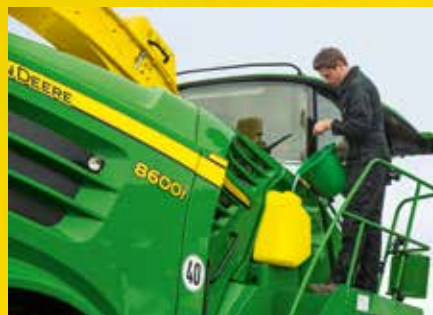
30 l concentrate tank
