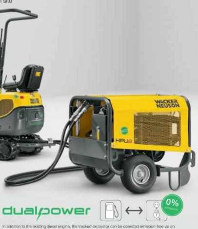
In addition to the existing diesel engine, the tracked excavator can be operated emission-free via ar electro-hydraulic power unit.
