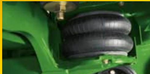
Air bags in front and behind the front walking beam help minimise impact.
