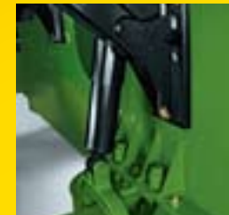
A heavy duty shock absorber provides additional cushioning.
