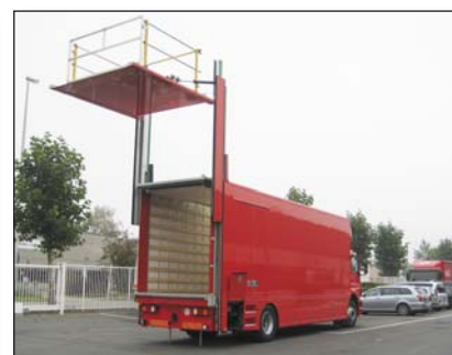
DH-VO5 1000-2000 kg - Lifting height up to 6 m above the ground
