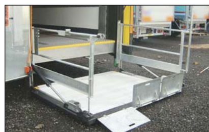
S751 Safety gates mounted to the lift runners instead of to the platform
