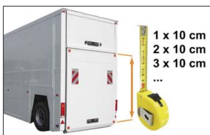
S714 Extension of the platform depth per 10 cm 1 x 10 cm 2 x 10 cm 3 x 10 cm ...
