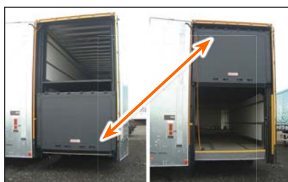
S730 Free passage of closed platform between different floor levels
