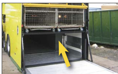
S728 Fixed platform without tilt cylinders (interior lift)
