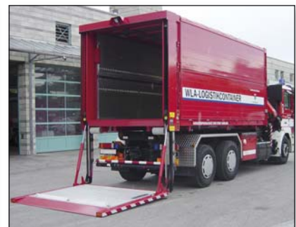
DH-VBC2 1000-2500 kg - Developed for containers & demount bodies
