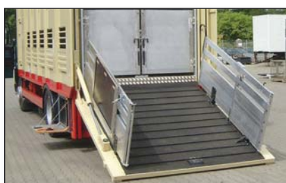
S709 Inclination of platform to the ground (max. 45°)
