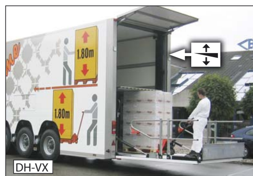
DH-VO5 1000-2000 kg - Lifting height up to 6 m above the ground
