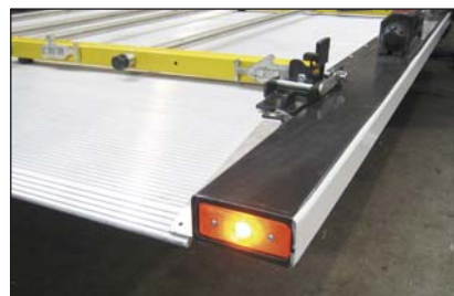
S708 Flashing lights mounted onto the platform point
