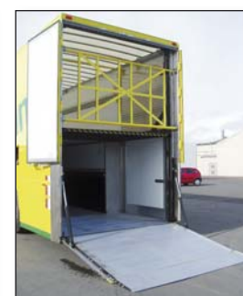
Interior DH-VX lift + exterior hydraulic ramp
