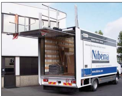
DH-VBA 750-1000 kg - Full alu lift with a reduced proper weight
