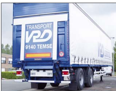
S201 Steel platform flat between the main beams
