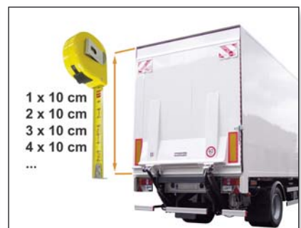
S203...204 Extension of platform depth per 10 cm : alu (S203) and steel (S204)
