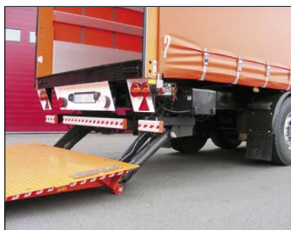
S362 3-piece bumper bar mounted to the lift frame
