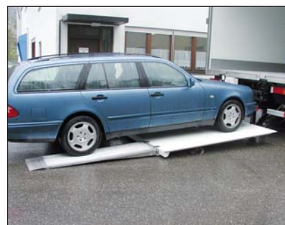
S239 Foldable cantilever platform
