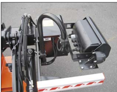
S411.LM Adjustable mounting bracket for the control box
