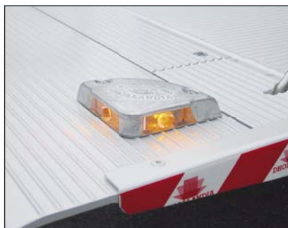
S090 Platform lights mounted onto the platform
