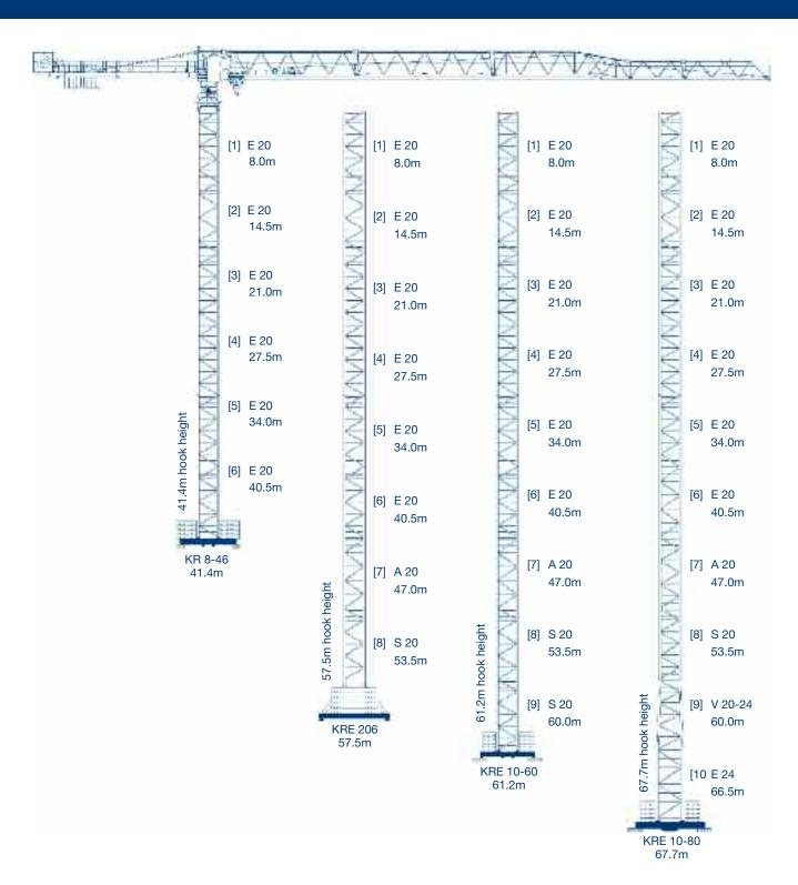
Tower combinations according to C 25 wind data. Lower under hook heights may be allowed for certain jib lengths.
