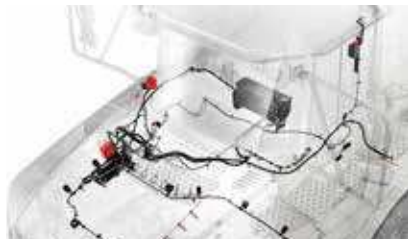
Fire suppression system
