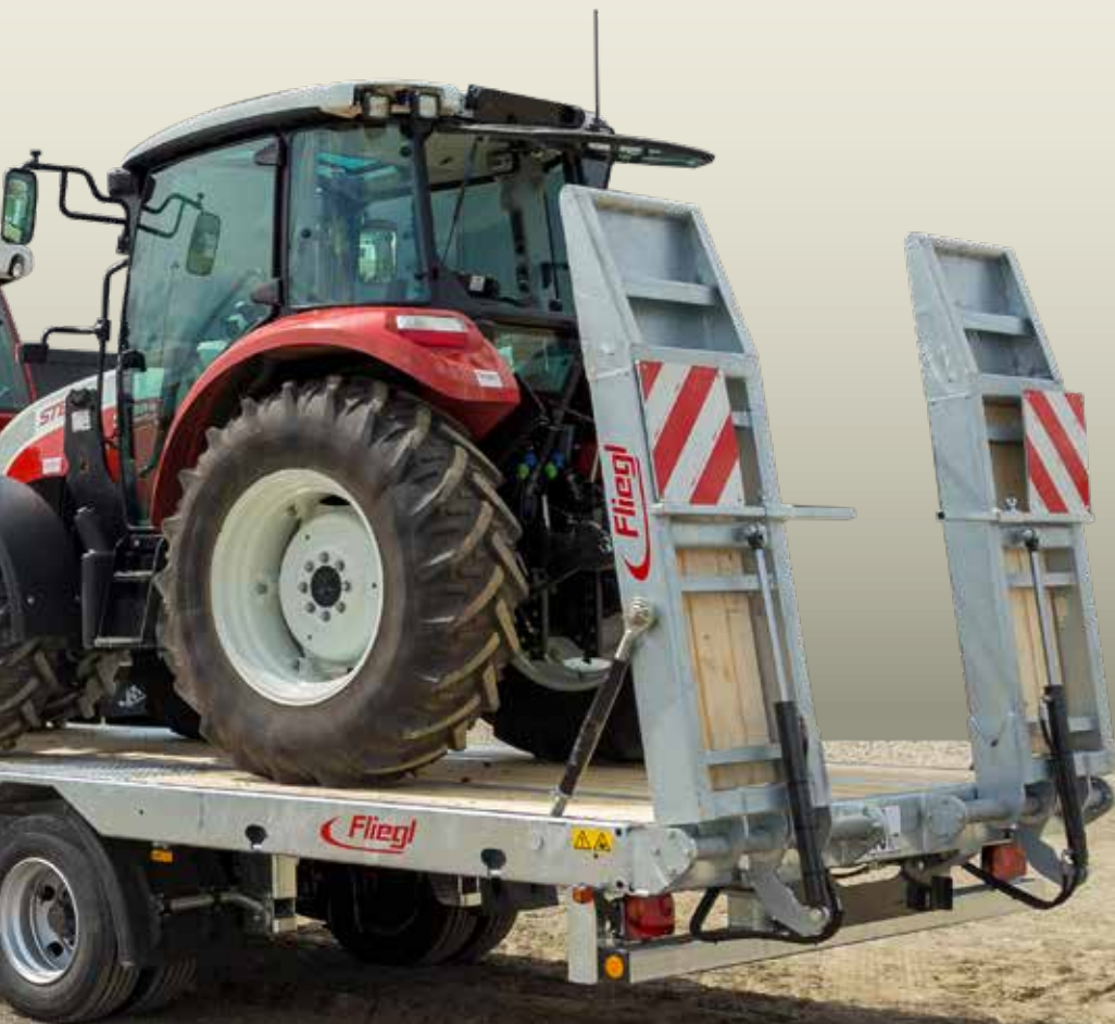
The TPA 370 Bulkhead 800 mm as standard Folding drive-on ramps
