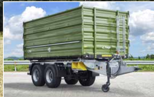
TDK 160 with 1800 mm body (3 x 600 mm tailgate)
