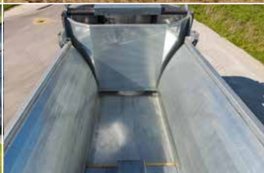
Minimum wear with hydr. pushing system - no scraper floor.
