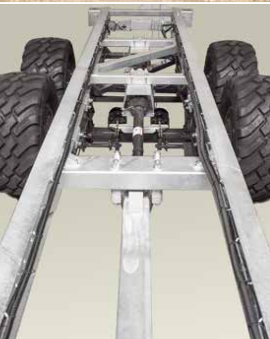
The spreading gear is driven mechanically by a PTO through-drive shaft
