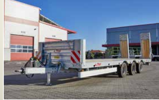
The TPA 370 Bulkhead 800 mm as standard Folding drive-on ramps
