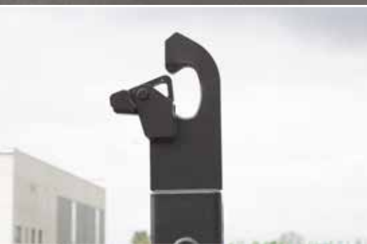
Forged, easily replaceable lifting hook
