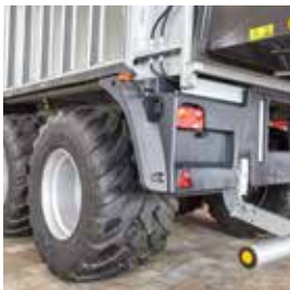
Mud guards and rear covers made of robust plastic parts guarantee clean surfaces and reduced risk of injury.
