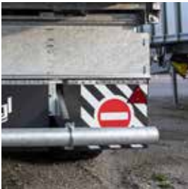
Germany 40 km/h version with fixed underride guard
