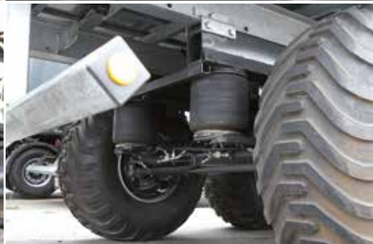
Optional: air suspension with automatic lowering when tipping
