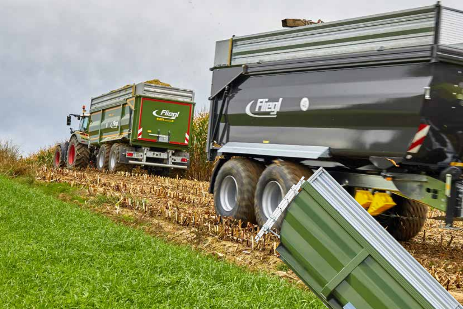
Tandem TMK 269 Profi with body length 6.90 m and tilt angle about 55°
