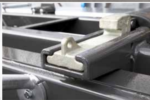
Reversible locking system for inside and outside locking
