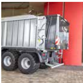
When the large-area back wall opens, the underride guard folds up automatically
