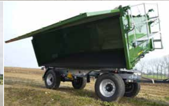
ZDMK 200 Profi with hydraulic opening side wall
