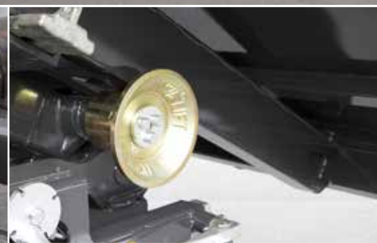
Large cast steel rollers ( \varnothing 310mm) with large centring bevel make it easier to raise the container.
