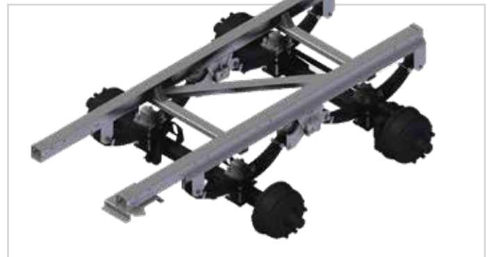
Gigant tandem assembly - parabolic suspension
