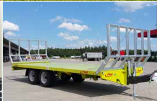
Tandem platform trailer with bale securing grid and special paint (optional)
