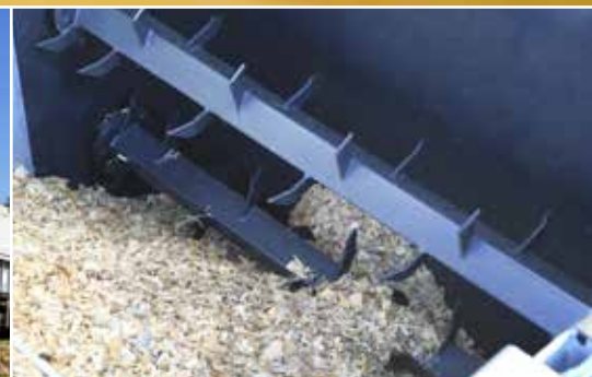
The milling drums ensure uniform feed
