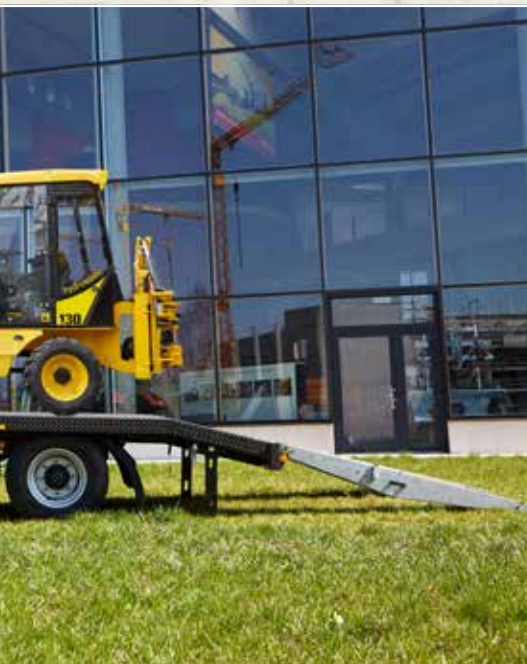
Drive-on ramps with wood covering, bridge floor made of 3.5 mm steel sheet, painted on the TPA 120
