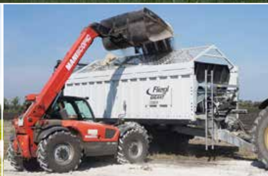
ASW 373 Tiger protective grating to protect from foreign objects
