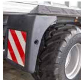
Mud guards and rear covers made of robust plastic parts guarantee clean surfaces and reduced risk of injury.
