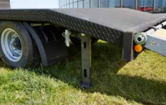
Top: drive-on ramps as standard with spring jack, and hydraulically operated as option
