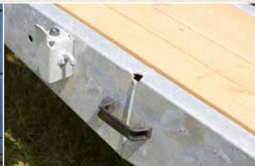
Drive-on ramps with wood covering, bridge floor made of 3.5 mm steel sheet, painted on the TPA 120
