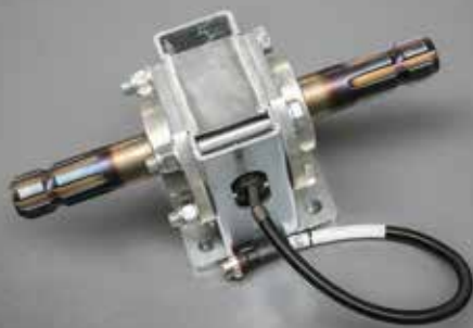
Automatic torque control with “I-SENS” feed control
