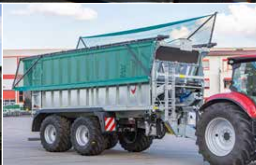
Cover net folds up to the side
