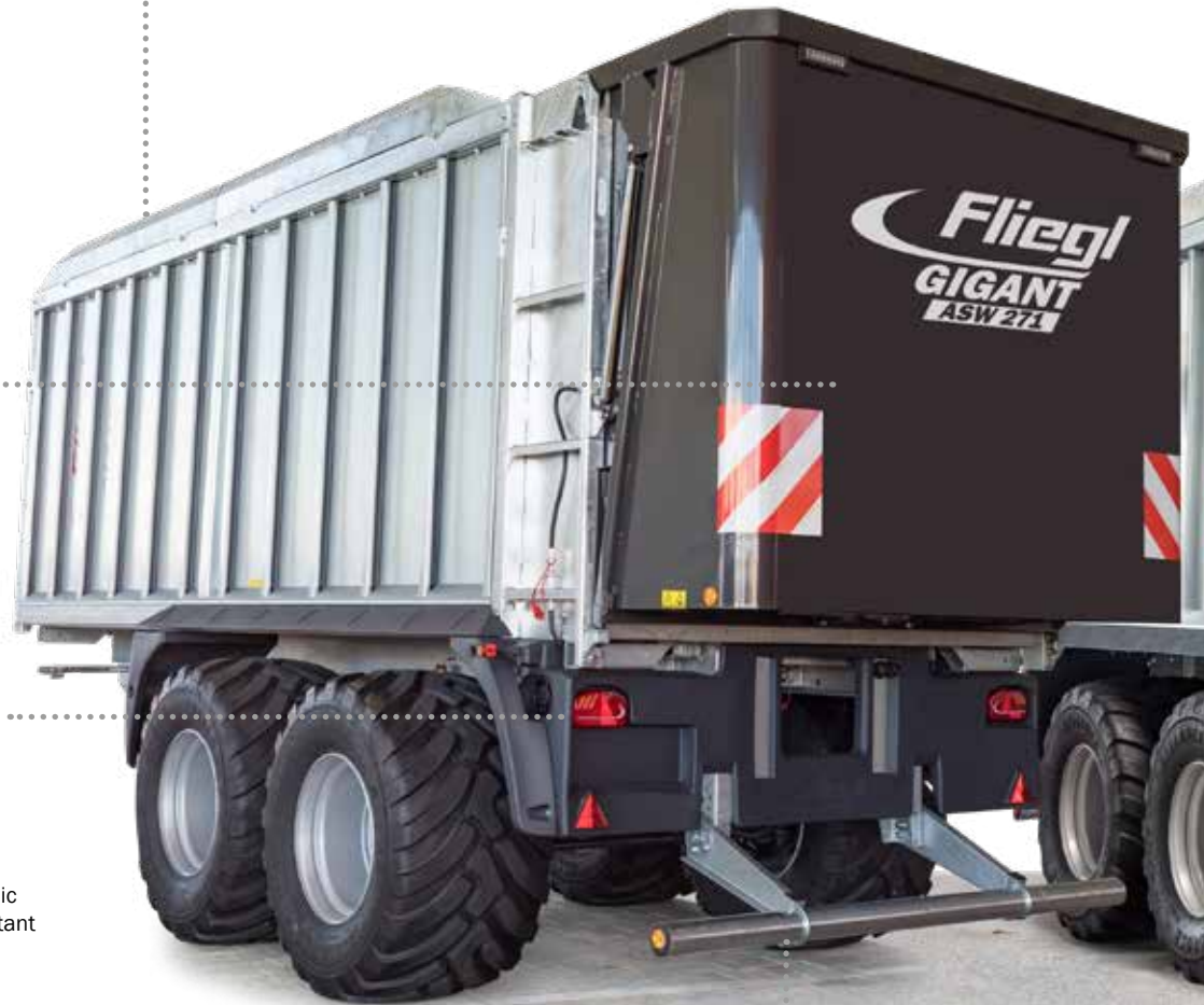
Hydraulic large area back wall
