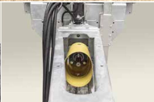
The spreading gear is driven mechanically by a PTO through-drive shaft
