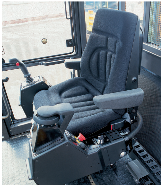
Sliding & rotating seat with integrated control instruments
