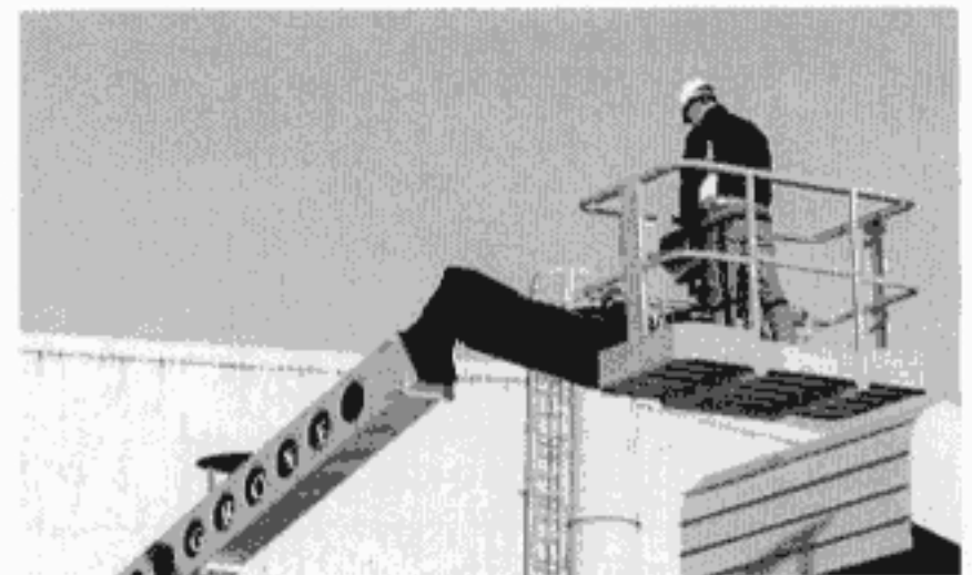
An articulating jib extension provides a third dimension for reaching around obstacles.
