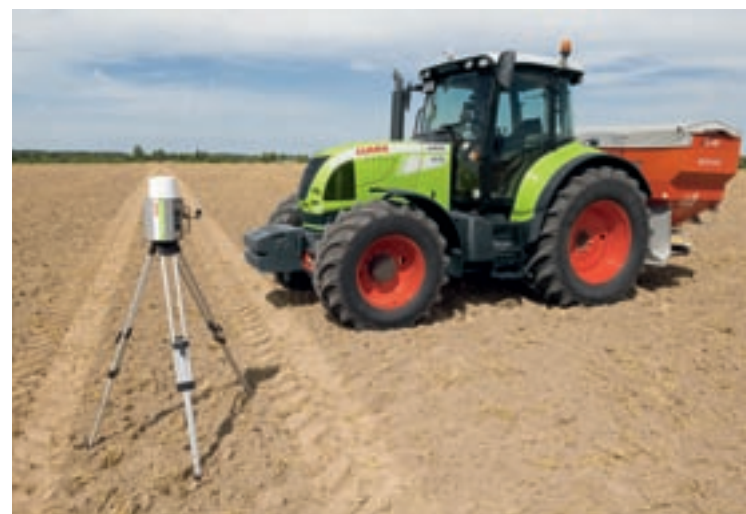
The GPS receiver on the BASELINE HD system. This includes an extra radio receiver for the reference signal.
