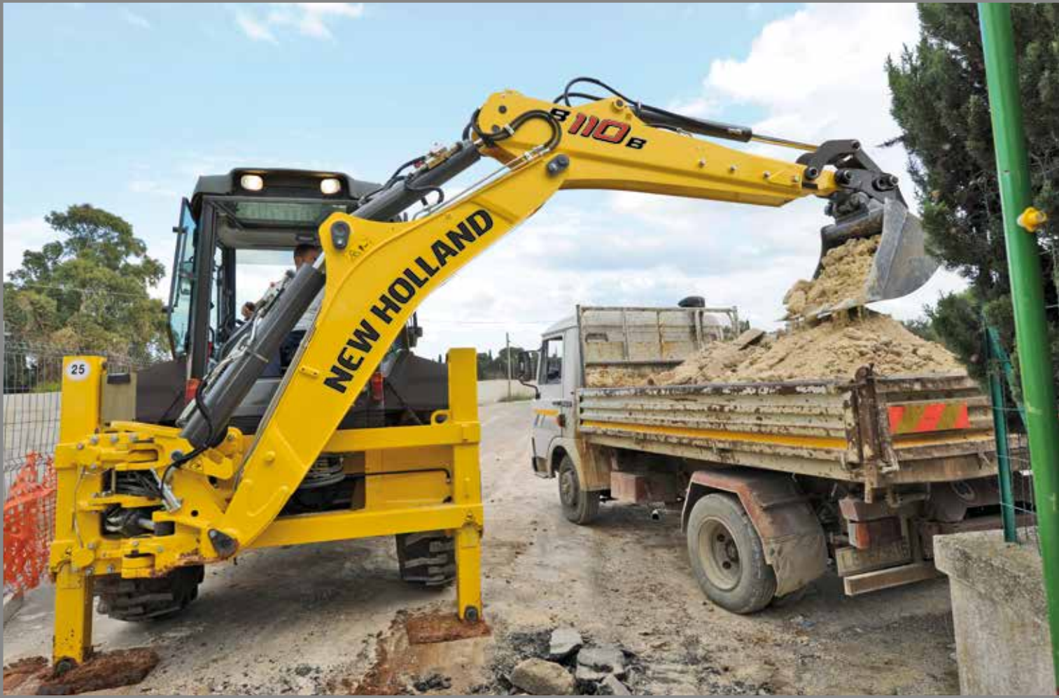
Thanks to the curved arm design, load sensing hydraulics and extensive backhoe reach
