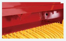
The replaceable feeder floor on all models provides wear resistance, easier serviceability, and extended baler life.
