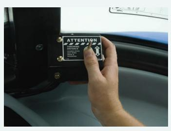
Distance and direction controller attaches to the tractor. The toggle switch controls the speed of the throwing belts for distance.
