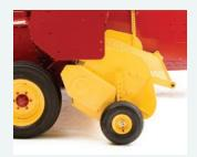
New pickup drive chain access shield provides easy entry for servicing. (Model BC5070)
