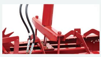
You can also equip your baler with hydraformatic bale tension control. This feature helps maintain uniform bale density in varying crop conditions.
