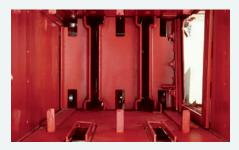
The rugged bale chamber is designed for better bale formation. Six hay dogs hold charges in place for firm, quality bales.
