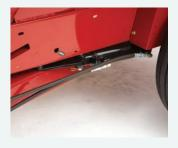
Hydraulic tongue swing uses hydraulic muscle to swing the baler into transport or working position quickly and easily.
