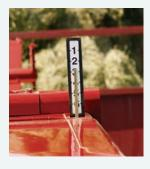
Distance Indicator is easily visible from the tractor seat. It shows you the relative distance bales are thrown, with "6" representing the fastest belt speed and furthest distance and "1" representing the slowest speed and shortest distance.
