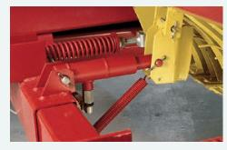
Hydraulic pickup lift. (Shown from rear of baler.) When baling, raise or lower your pickup as needed to adjust to differing terrain without leaving your tractor seat.
