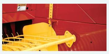
Pickups are manually raised and latched into transport position. Hydraulic pickup lift simplifies raising and lowering the pickup. It's standard on the BC5070 Hayliner and optional on other models.
