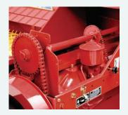
Hydraformatic oil pump is conveniently located for easier serviceability. (Models BC5060 and BC5070.)
