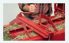
Tension springs are the economical way to adjust bale tension. A one-half-inch increase in spring tension equals 600 pounds of increased force.
