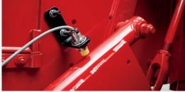
The automatic CropSaver applicator with stroke counter utilizes position sensors to detect when each bale is tied, the number of strokes per bale and determines the tons per hour harvested. Displayed on the monitor, this information allows the operator to adjust baling speed to maximize productivity and maintain an accurate bale length.
