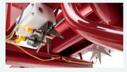
The automatic CropSaver applicators feature twin star wheels mounted on the underside of the bale chute that measure the moisture in each bale and continuously adapt the application rate every three seconds to respond to moisture changes.
