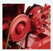
Redesigned knotter gear drive makes servicing or replacing the pickup belt simple.
