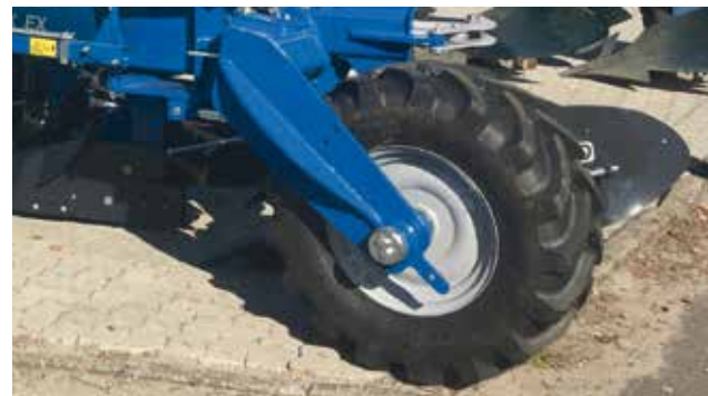
Tractor treaded support wheel - 320/65x16 EX, VFEX, VFEX On-land. Mechanical depth control, and damping with friction brake.
