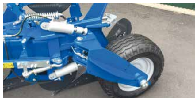
Hydraulic depth control for combi-wheel above
