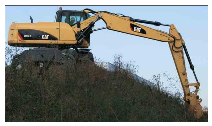
**Design.** Booms and sticks are welded, box section structures with thick, multiplate fabrications in high stress areas, for rugged performance and long service life.
