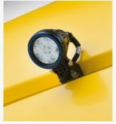
• Rear lamps enable operators to monitor residue and two lamps located on the side panel illuminate the rear axle to prevent crushing standing crop and to assist when manoeuvring
