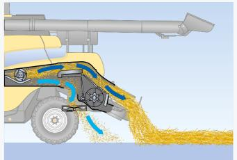
• The high speed chopper, 3500rpm on CR7.80 to CR8.80 models and 4000rpm on CR8.90 models and above, ensures fine chopping
