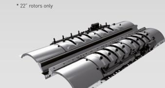
The rotor vanes can be remotely adjusted so that optimal crop threshing efficiency is maintained, even when crop conditions change. This enables overall capacity increases of up to 20%\*.
