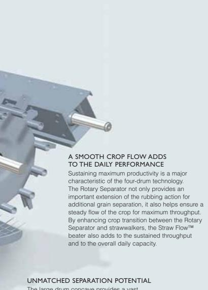
The large drum concave provides a vast separation surface. The concaves under the beater and the Rotary Separator add more powered separation area. The beater, the Rotary Separator and the Straw Flow™ beater each create a directional change in the crop flow, increasing grain separation. For higher straw quality in crops that do not require the extra rubbing, the four-drum technology includes the Multi-Thresh™ system that can lower the concaves of both the beater and the Rotary Separator.
