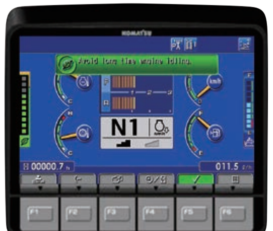
Eco gauge, eco guidance and the new auto idle stop help to further reduce consumption.
