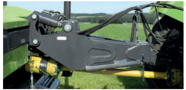
The bottom-mounted drawbar is available as standard.
