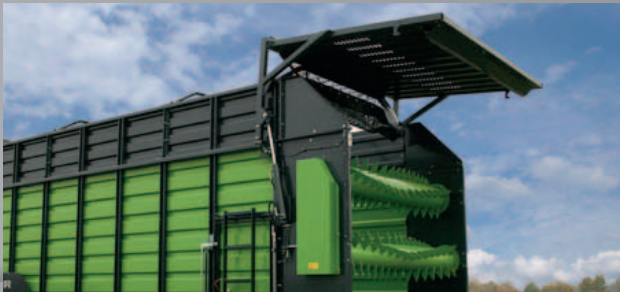
The opening angle can be set manually.
