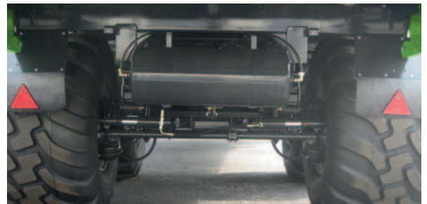
Air brake system for safe transport is available as option.
