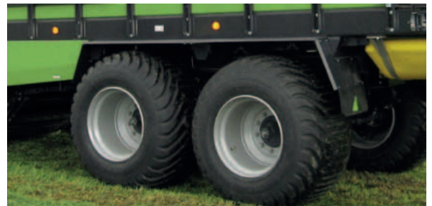
Large 600/55 - 22.5 tyres are standard fitted on RotoMaster 5520.
