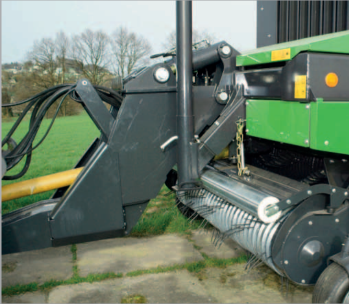
The RotorMaster models are as optional fitted with hydraulically articulated pin-hitch drawbar.
