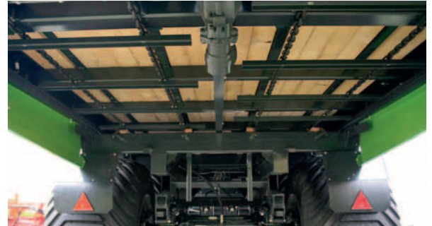
Chain-and-slat conveyor with split driveline and gearbox positioned in the middle.
