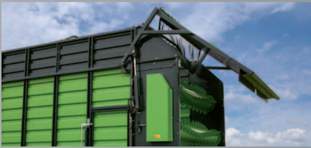
The sensor controlled tailgate.
