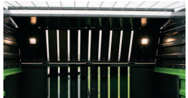
The deflector plates ensure optimum distribution of the crop throughout the entire chamber.
