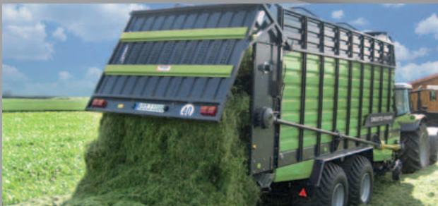
The speed of the chain-and-slat conveyor is infinitely adjustable.
