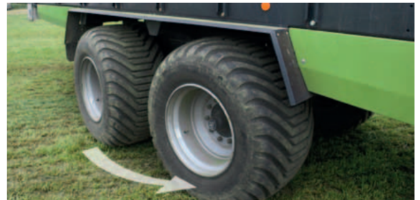
Actively steered wheels for improved manoeuvrability.
