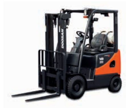
G15S / G18S-5 & G20SC-5 1,500kg 1,750kg 2,000kg LPG, Pneumatic Tire
