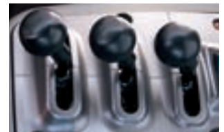
Fingertip control 3 levers control for lift arm, bucket and 3rd circuit. FNR switch for changing travel direction as well as kick-down, return to dig, lift arm raise kick-out and floating mode.
