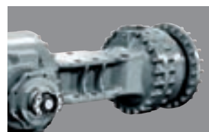
Differential hydraulic lock For automatic (depending on transmission torque) or manual differential lock (optional on DL450-3).
