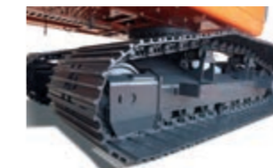
High track (on DX160LC-3) Ideal in forestry, recycling and demolition due to its higher ground clearance (15 cm).
