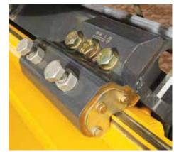
Jackscrew adjusted sideshift wear inserts keep the moldboard tight and precise. Takes only minutes to return tolerances to factory spec.
