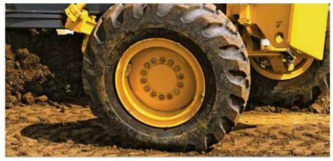
Power is nothing without control. On our six wheel-drive graders, the front wheels engage smoothly and in sync with the rear tandems - making them highly adept at finishing.
