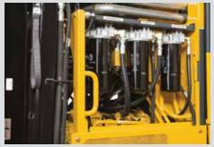
Maintenance personnel will appreciate the unique easyaccess hydraulic, transmission, and differential filter bank.
