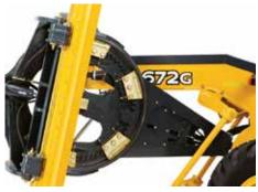
High-strength circle and draft frame with stand high-impact loads. Available blade impact system further protects structural components from damage caused by run-ins with obstructions. Blade is prestressed for exceptional strength and durability.
