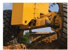
Front axles are built to last with exclusive heavy-duty tapered roller bearing king pins. In addition, steel guards and thick rubber coverings protect the hoses on sixwheeldrive models.
