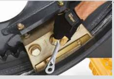
Two-hour replaceable supertough nylon or bronze draft frame and circle wear inserts minimise maintenance labour.
