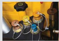
Optional quick fluid servive ports help speed servicing. 500-hour engine oil/filter; 2,000-hour transmission, hydraulic, axle filters; and 4,000-hour transmission, hydraulic, axle oil service intervals minimise maintenance.
