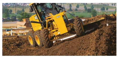
Steering system automatically adjusts the speed of the outside front tyre while increasing pull to provide full power turns.
