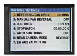
Reversing fan automatically cycles at predetermined intervals, ejecting debris from the radiator and cooler cores. Or choose your own cleaning cycles through the monitor.
