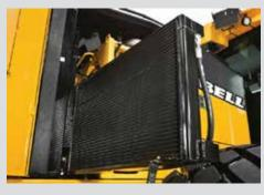
Exclusive cooling package features stacked coolers that swing down and a hinged rear fan that opens out of the way for easy cleaning. Takes only seconds to gain access to the cores.
