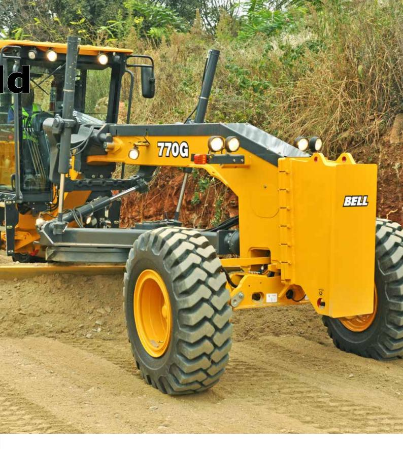
Best-in-class lever efforts are combined with Pressure-Compensated Load-Sensing (PCLS) hydraulics to ensure consistent, predictable, and precise response. Automatic differential lock stays engaged when travelling straight, disengages in turns exceeding 10 degrees, and re-engages when returning to straight.
