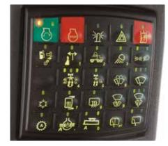
Sealed-switch module provides pushbutton control of 25 machine functions including keyless start. When enabled, keyless start requires a numeric pass code that helps prevent unauthorized machine operation.
