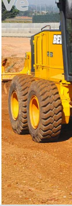
Six-wheel drive enables these graders to work across steep slopes, carry big loads through corners, and direct the front wheels while ditching without spinning out.
