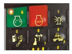
Switch module and electrical centre employ circuit-board technology that reduces connections from 25 to 1, and wires from 100 to 4. Solid-state sealed switches keep out moisture, debris, and are proven reliable for more than two million cycles.
