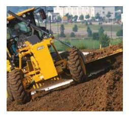
Exclusive ball-and-socket draft-frame pivot and seven-position saddle provide best-inclass blade setup and improved ditch cutting, ditch cleaning, and reach outside the tyres.
