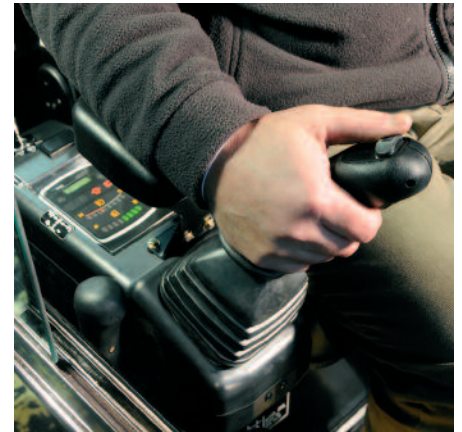
Well-appointed operator's station with thumb-operated proportional boom swing and auxiliary hydraulic functions.
