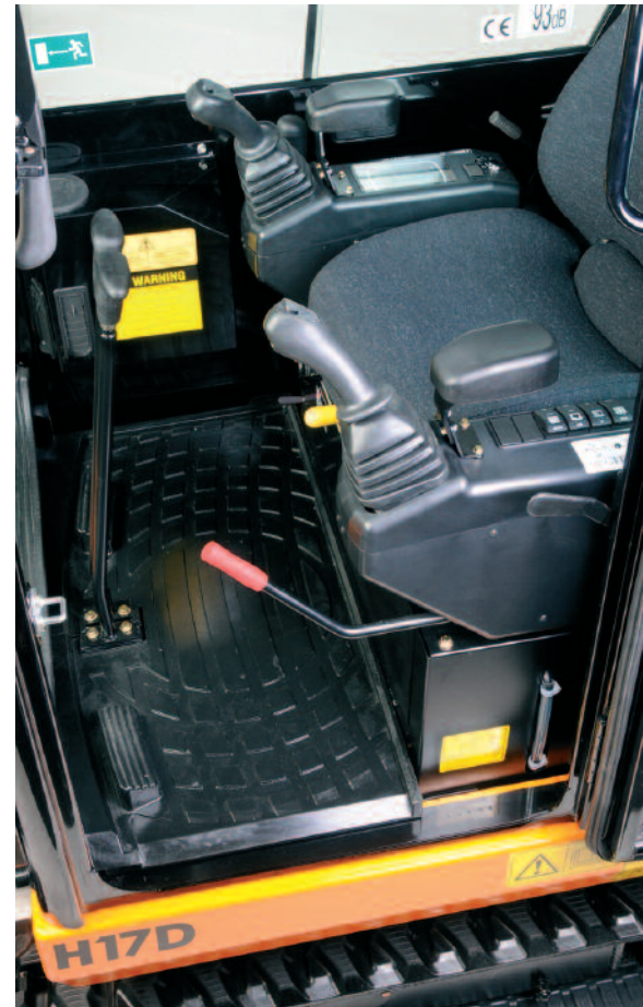
Spacious and comfortable cabin with a steel-framed door. With no curved glass on the machine, glass replacement is simplified should the need arise.
