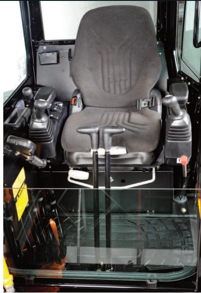
Spacious and comfortable cabin with a steel-framed door. With no curved glass on the machine, glass replacement is simplified should the need arise.
