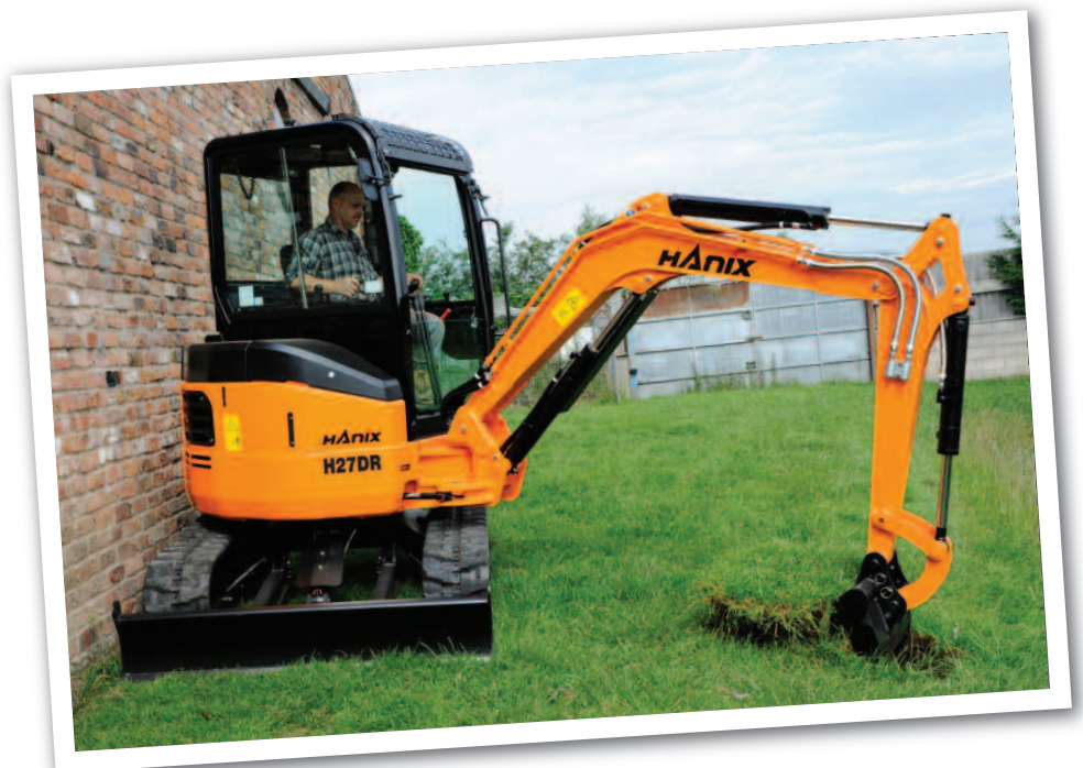
The zero tail swing design ensures maximum productivity in space restricted areas enabling the machine to work tight to boundaries and structures.
