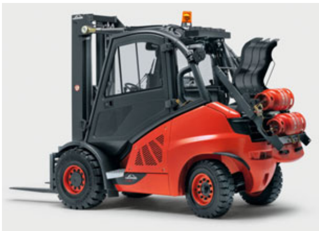
Ergonomic bottle replacement in LPG operation. No unnecessary force required from the driver.
