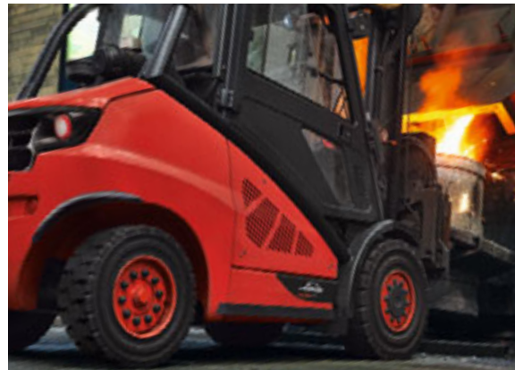
Designed for use in the toughest environments. Linde truck in heat-resistant foundry design .
