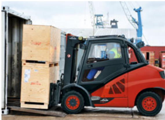
Ideal for low entrances. Even for the powerful 5-tonne trucks, Linde offers a version with a height of just 2.22 m.
