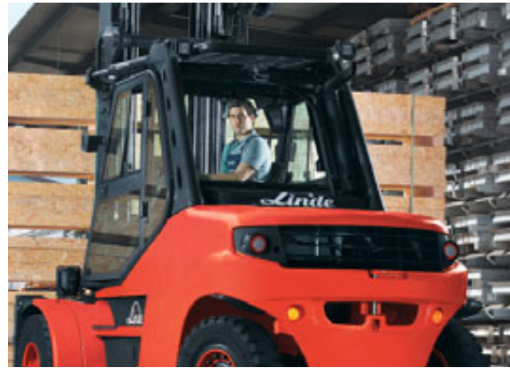
Rotating driver's workstation with fully rotating pedals and operating devices. Whether travelling forwards or backwards, with a slight head movement the driver has the load and route in view.
