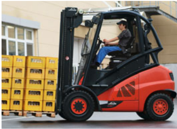
Linde truck in beverage industry version. The driver has a good view from the raised cab at all times – even if loads are stacked high on the fork.
