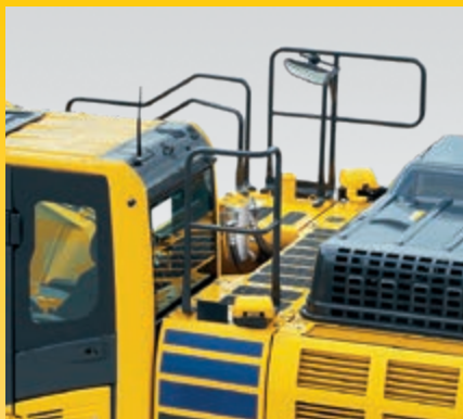
Hand rails and anti-slip plates
