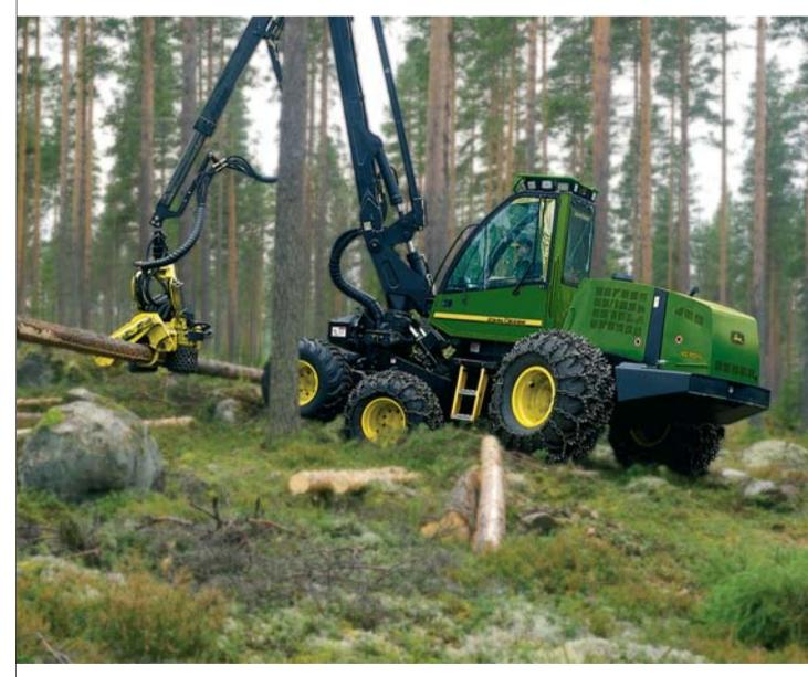
Super-efficient, electrically controlled common-rail fuel-injected John Deere engines achieve high torques of 498 Nm (770D) and 779 Nm (1070D) at very low rpm. This leads to lower fuel consumption and a lengthened life for the components.
