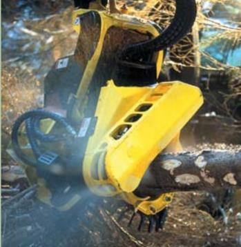
The new, extremely accurate feed control based on the Timbermatic 300 provides power and speed for delimbing. The increased working pressure of 28 MPa in the 1070D prevents skidding and improves the quality of work even further.
