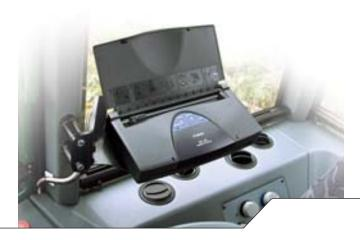
The Timbermatic 300 features a versatile fault diagnostics function and the system issues reminders of scheduled maintenance services. The reports can be printed out as A4 size sheets.
