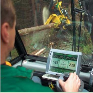
In addition to volumes and measurements, the PC-based Timbermatic 300, which runs on a Windows operating system, collects information on the location of produced timber, which can be sent to the forwarder or the factory in order to optimise transportation. Starting a new site is easy. Map information, as well as site and felling instructions, is transferred directly to the system via a wireless connection.
