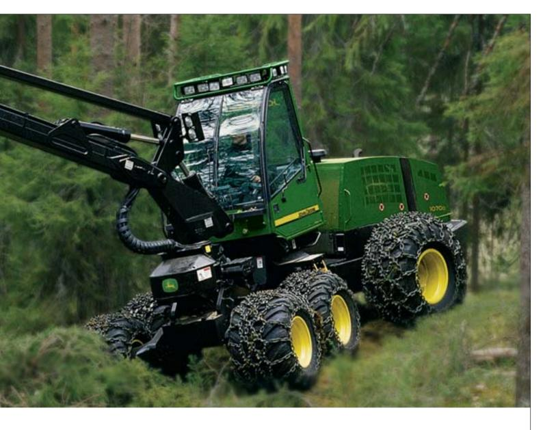
The strongly built parallel booms are positioned on the front frame of the machine practically parallel to the field of vision of the operator. This allows for smooth and natural controlling of movements in all directions. The boom can be tilted backwards by 15 degrees and forwards by 15 degrees (770D) or 23 degrees (1070D), either manually or automatically. The automatic tilting feature improves working in demanding conditions.
