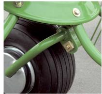
**The eccentric adjuster** Setting the angle of throw from 14° to 19° is easy and fast using an eccentric ring on the wheel assembly.
