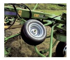
**Spare wheel** Stored on a holder supplied with the wheel, the spare is easy to remove without tools.
