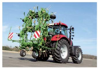
Safe travel on the road KW 11.22 folds into a compact storage 'package' (3.75 m (12'4") high). Its 2.98 m (9'9") transport width makes road travel a safe and relaxed affair.
