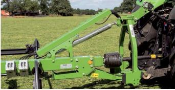
Another option (the 'Plus' design) is the three-point hitch system, which offers advantages in tight turns and headland turns. The sward is protected, too, as the weight is shifted actively from the chassis to the rotor wheels (option).
