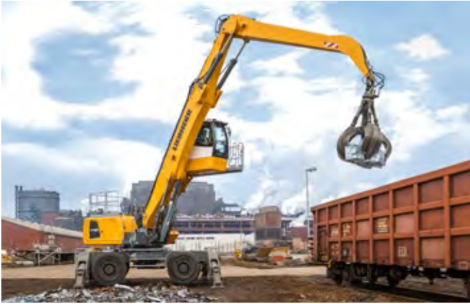
Loading extruded aluminium bundles onto wagons with the LH 50 M Industry Litronic
