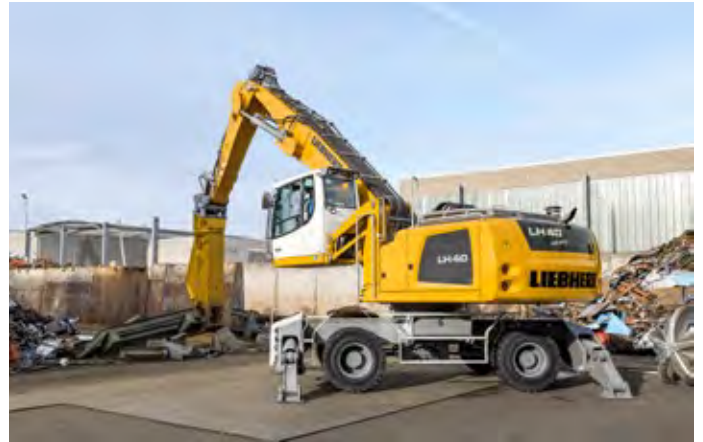
LH 40 M Industry Litronic for disassembling steel girders with a scrap shear
