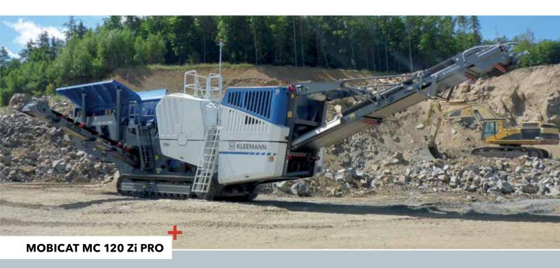
The MOBICAT MC 120 Zi PRO, the first jaw crusher in the PRO line, is used for pre-crushing of almost all natural stones. The jaw crusher has an extremely robust design and impresses with its low-maintenance operation. The machine therefore guarantees high production outputs.
