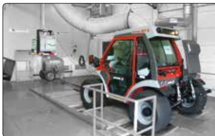
Before delivery, all vehicles undergo intensive functional testing such as here on the roller test bed.
