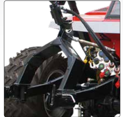
The Metrac H4 X has a front linkage with integrated lateral displacement.
