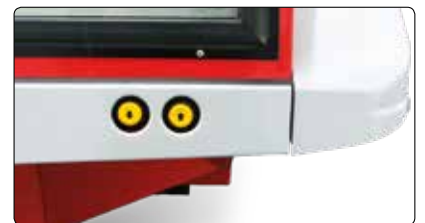
The exterior electric control for the front linkage is standard and makes mounting of attachments much easier.
