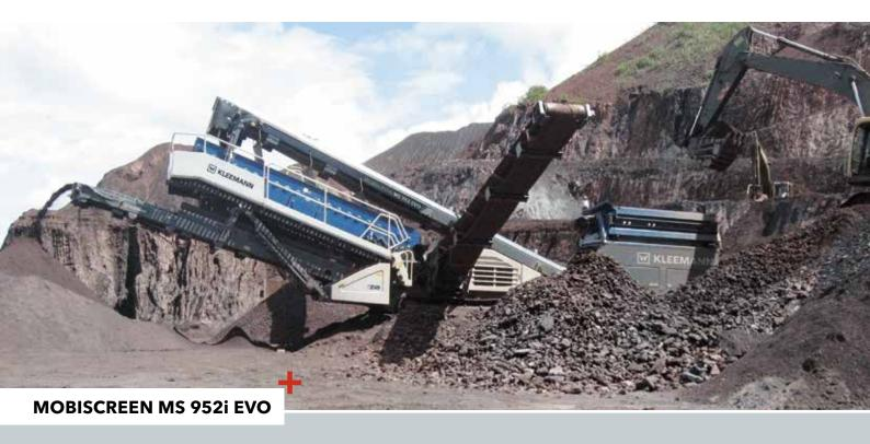
As a double-deck classifying screen, the mobile screening plant MOBISCREEN MS 952i EVO is equipped with a  $9.5 \text{ m}^2$  screen casing. The plant impresses with a feed capacity of up to 551 US t/h. It is controlled using a modern control system. As a result, all functions are easy to control and operating statuses and machine functions can be viewed at any time.
