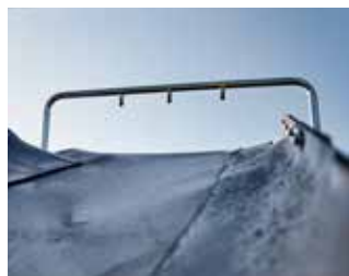
Water spraying system for efficient dust suppression, pump included
