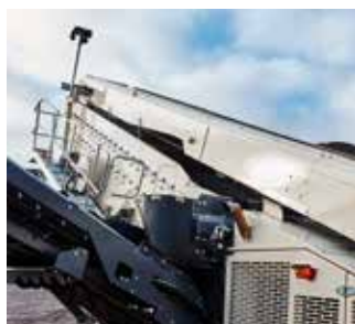
Hydraulic raising of lifting conveyor as standard, to allow more space for maintenance
