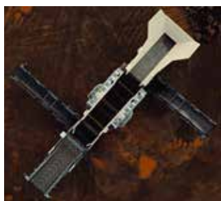
Large screen box with 10 mm stroke for efficient material separation
