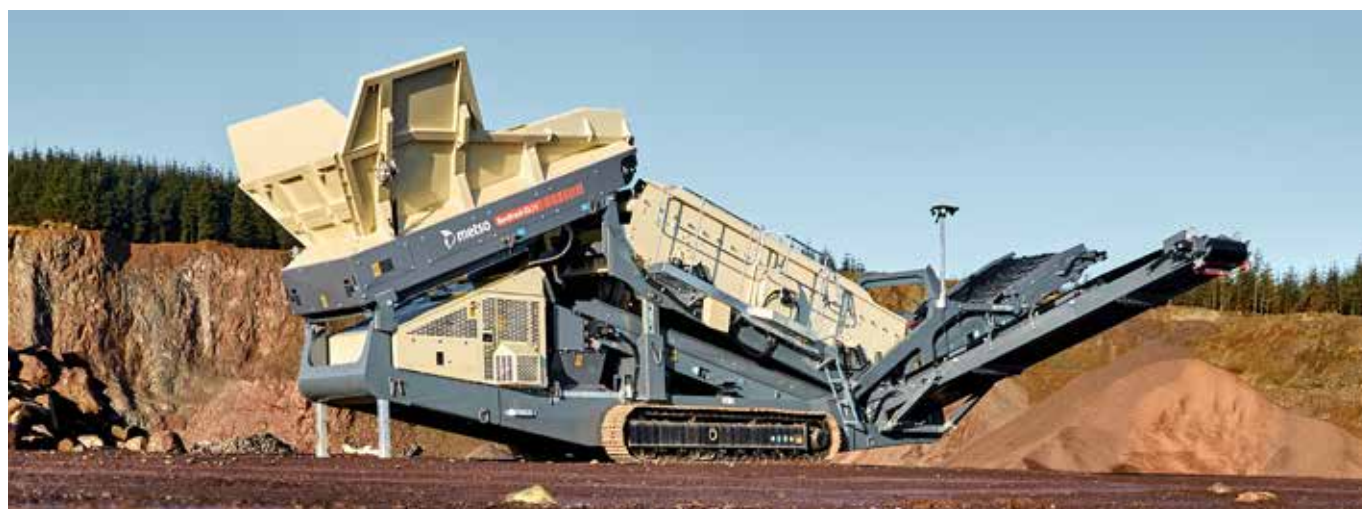
Six emergency stops, start siren, engine shutdown system and nip point guards for safety
