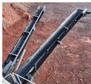
Heavy-duty chevron belts for lifting, oversize and side conveyors for maximal durability
