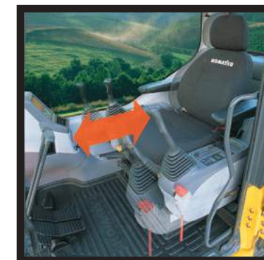
Seat Sliding Amount: 340 mm 13.4", increased 120 mm 4.7"
