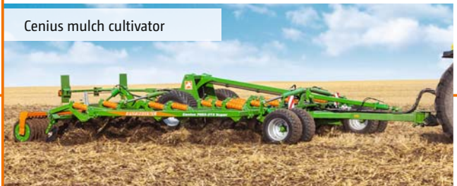
2 nd pass: Working depth approx. 10 cm
