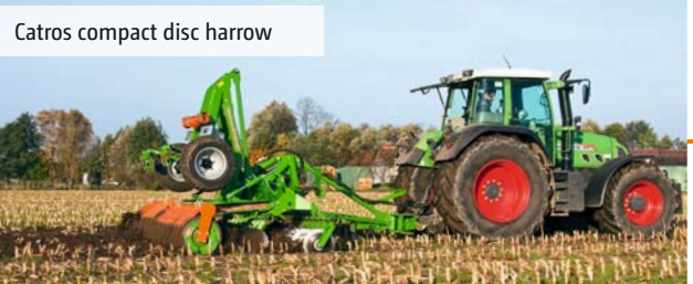
1 st pass: Working depth approx. 5 cm
