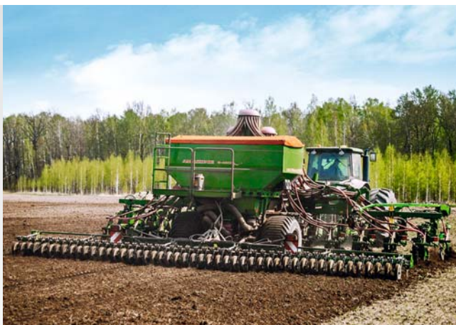
Primera DMC, 9 m working width, “RL Brjansk” farm
