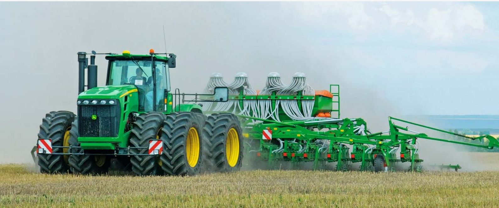
Primera DMC, 12 m working width
