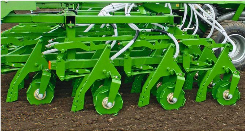
The coulters units are arranged on longitudinal cross members in 4-stagger which results in a large distance from one to the other, and thus good straw passage.
