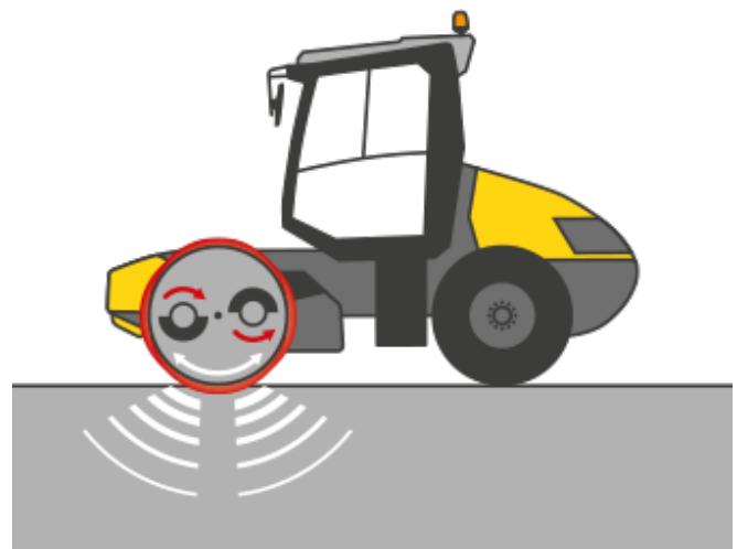
Compaction type 2: Oscillation for optimal surface compaction.
