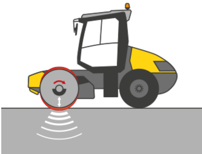
Compaction type 1: Vibration for high compaction depth.
