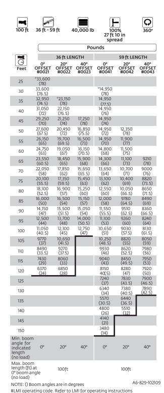
\*This capacity is based on maximum obtainable boom angle.
