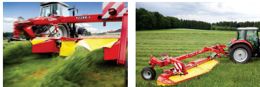
Edge mowing (mower angled at 25°)
