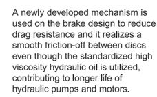
With a new negative brake of spring-applied/power hydraulically-released design applying dynamic hydraulic pressure for its release control, an effective braking can be done under an extreme light foot pedaling, and it accordingly results in greatly reducing operator fatigue especially during winch free-fall operations under duty cycle applications. Further, the use of negative brake system maintains a high level of brake safety even if a hydraulic pressure drop in the circuit happens.
